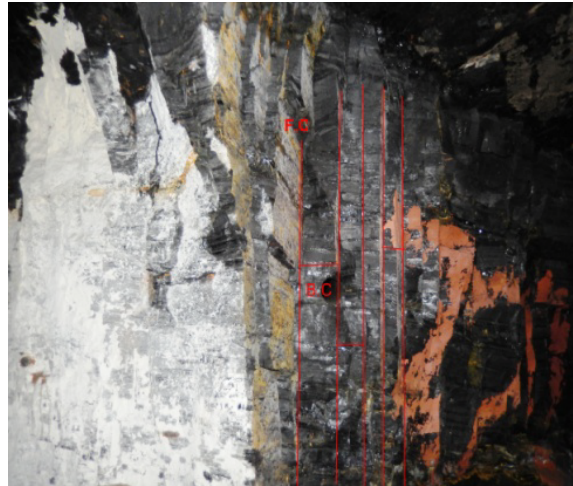
Photograph 3 Face Cleat & Butt Cleat in Coal Pillar
