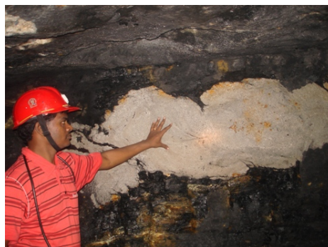
Photograph 1 Sandstone intrusion in coal pillar
